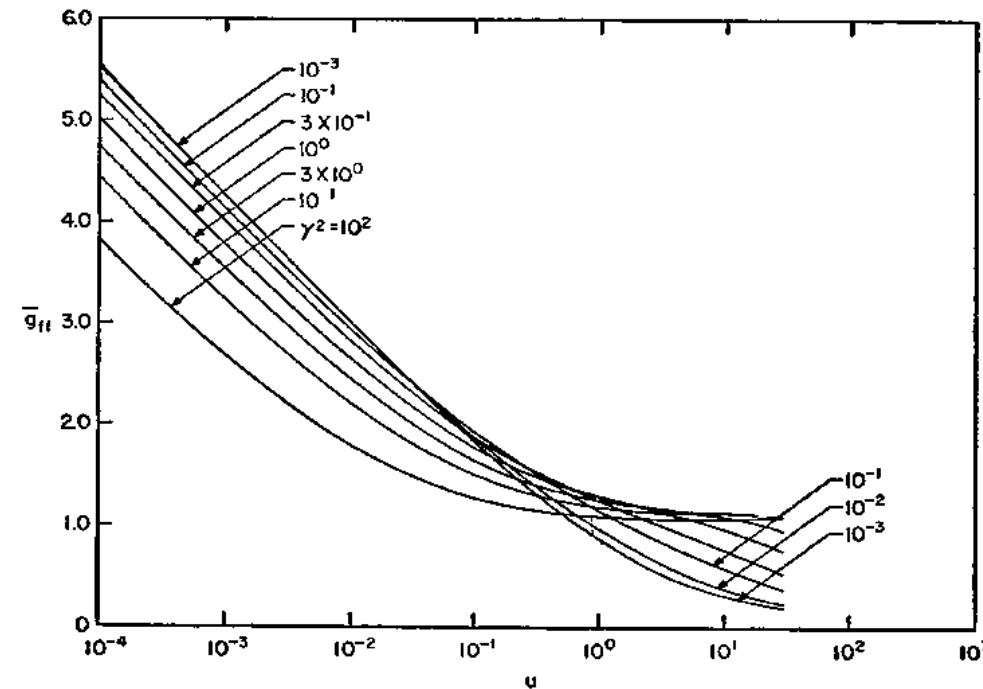
Gaunt factor,  $\bar{g}_{ff}$ , from Karzas & Latter, Fig. 5.  $u = h\nu/kT$ , for various values of  $\gamma^2 = Z^2 \text{Ry}/kT$ , where 1 Ry = 13.6 eV.
